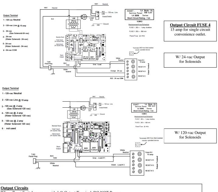
Where Reset Switches are provided @ Output Terminal, DO NOT Bypass.
